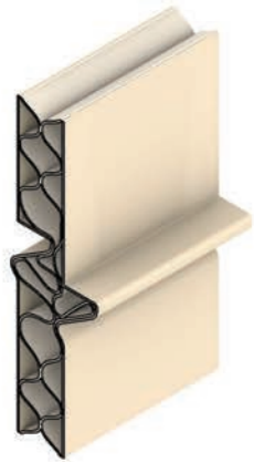
Figure:4.H Reactive inner and outer skin Parallel loading
