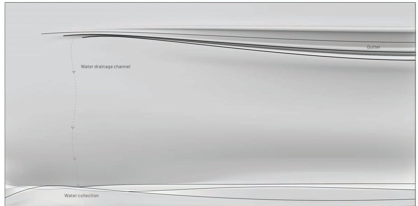
Figure:5.D Gutter elevation 1:20
