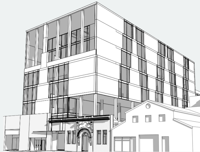
Figure 6. 3D visualisation of the stretch scenario with a window-to-wall ratio of 40%.
